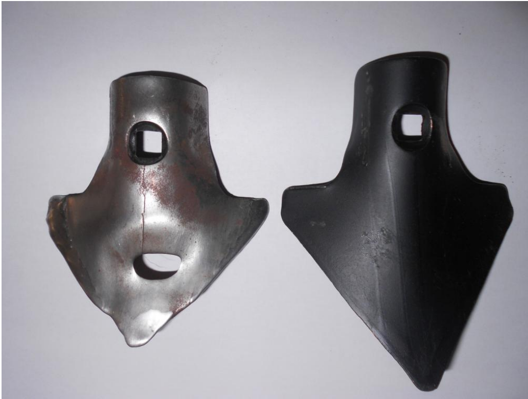
Figure 2 A new and a worn out „flat feet” hoes
