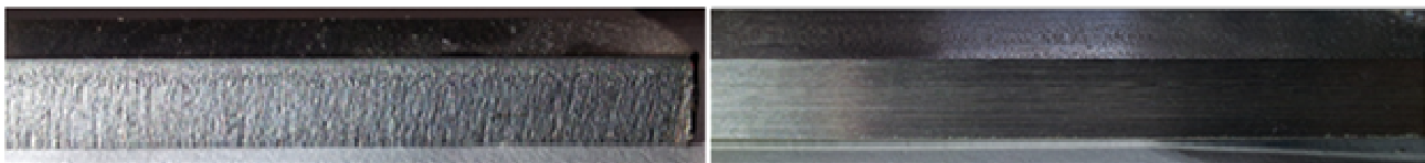
Figure 2 Material cut by the means of plasma beam (left) and with band saw (right)
