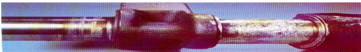
Figure 3 Typical deterioration,an cranckshaft submissive washing with oil by refrigerant
