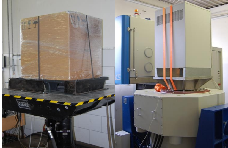
Figure 6 Hydraulic and electrodynamic vibration system with packaging testing purposes [7]
