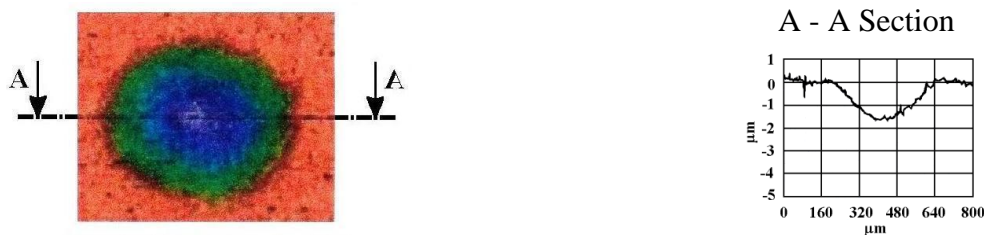
Figure 3 Depth of remaining crater on TiN/ SS316L determined by measurements of confocal 3D microscopy (left) and profilometry (right), depending on the duration of the impact
