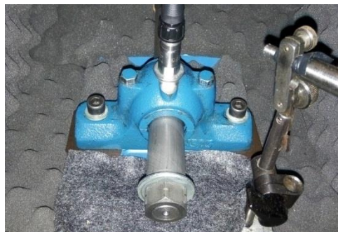
Figure 2 Test rig for tapered roller acoustic chamber
