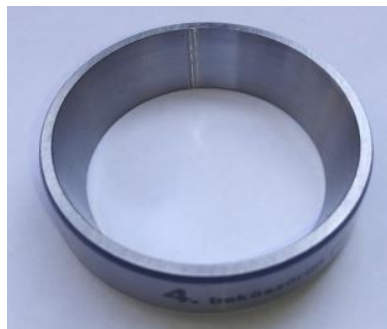
Figure 3 Outer ring of the tapered roller bearing with grinding defect of 1.6236 mm
