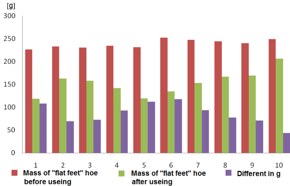
Figure 6 Mass changing of spray fused hoes in g before- and after using
