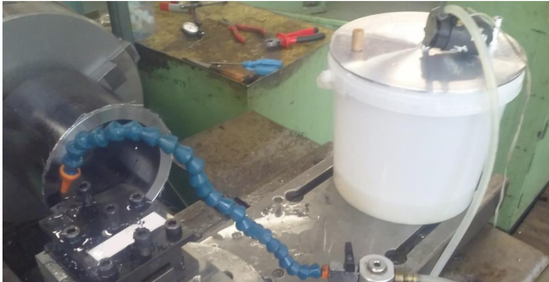
Figure 3 The supply of the cutting emulsion into the place of cutting
