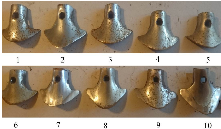
Figure 8 The experimental workpieces after use. Heat-treated pieces (upper row) and the sprayed pieces (bottom row)
