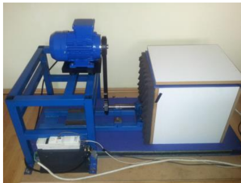
Figure 1 Test rig for tapered roller bearing measurement
