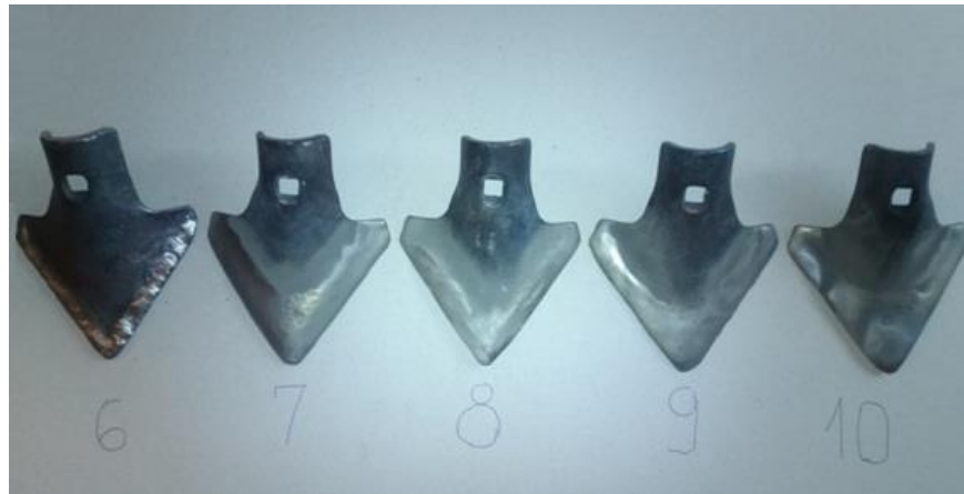
Figure 5 Spray fused „flat feet” hoes
