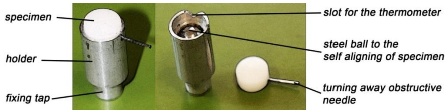
Figure 3 The fixed specimen holder and his main parts
