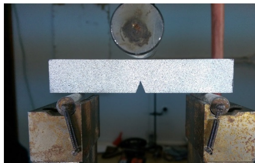
Figure 3 The prepared specimen, prior to loading
