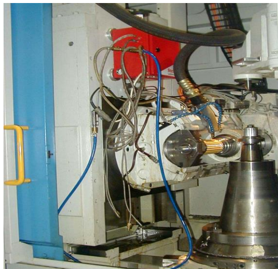
Figure 21 Environmental lubricant devices on Pfauter PE-500 CNC milling machine
