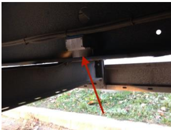
Figure 3 Data logger (SAVERTM 3X90) used in this study (right picture source Lansmont brochure, lansmont.com)
