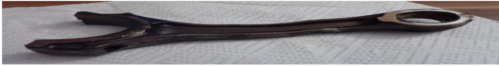
Figure 9 Damaged piece-winch from an overheated compressor
