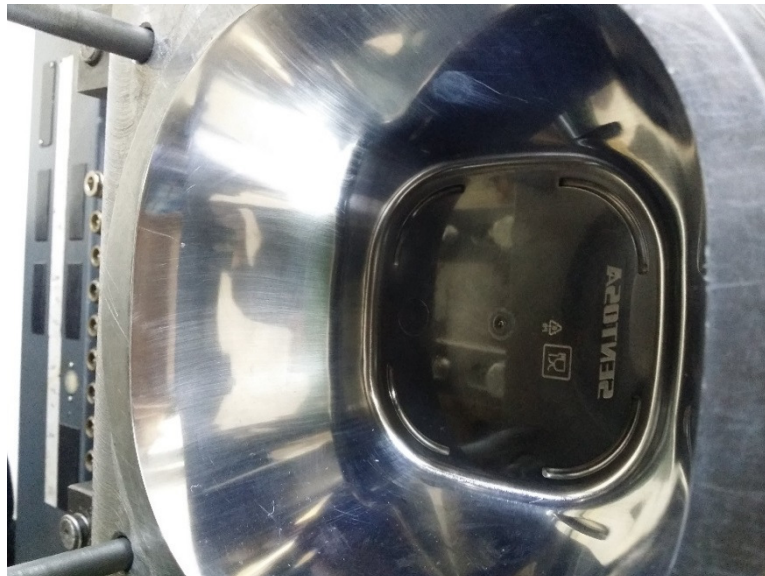
Figure 4 Surface after re-machining with abrasive tool in a slope angle of 20 degrees
