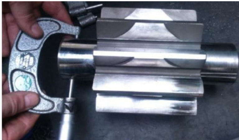
Figure 2 Measurement of the A dimension on the driven sprocket [8]
