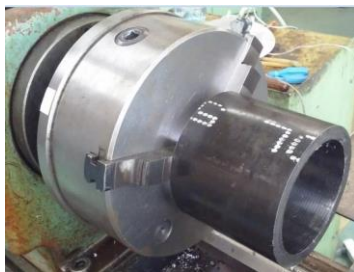
Figure 2 Clamping of the workpiece – pipe and dynamometer Kistler 9257B
