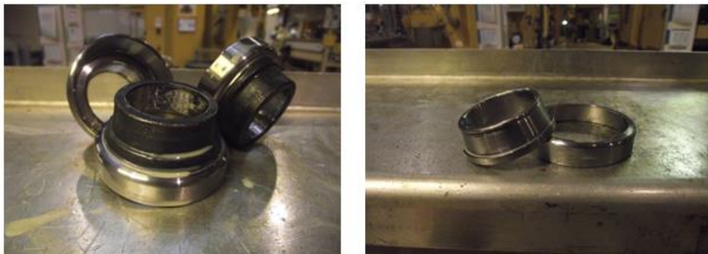
Figure 2 Laterial grinded tower ring (left) and separated rings (right)
