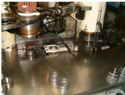
Figure 8 Stamping and pulling of the cage (left) and construction operation (right)
