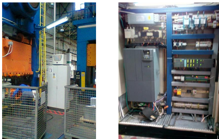
Figure 5 Closed press frame; Electric panel with frequency converter
