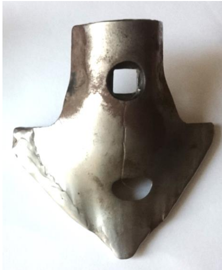
Figure 2 Worn cultivator tine
