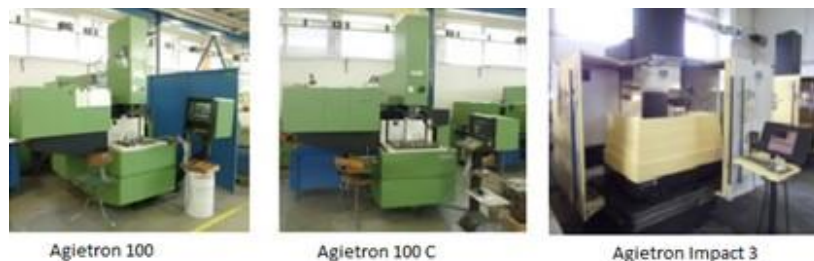
Figure 3 AGIE die-sinker EDM machines applied in the experiment
