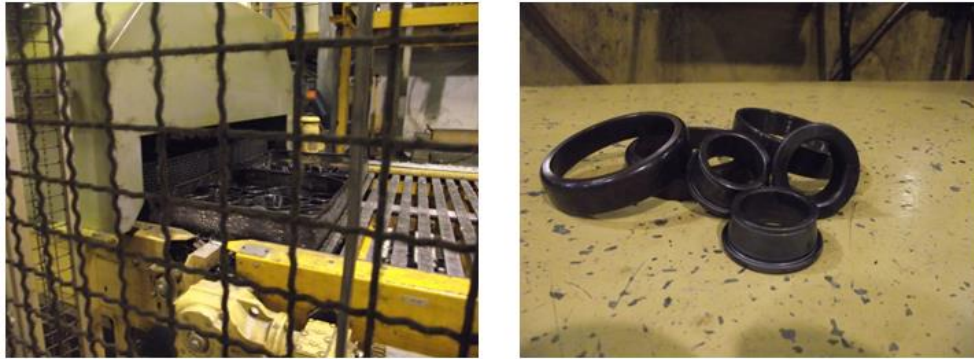
Figure 3 Heat treatment furnace (left) and heat treated rings (right)
