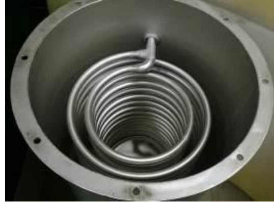
Figure 4 The double pipe coil inside the tank
