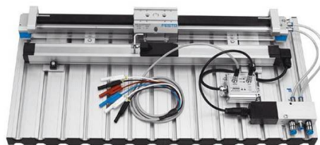
Figure 3 DGPL-25-450 Pneumatic cylinder with attached encoder and servo valve
