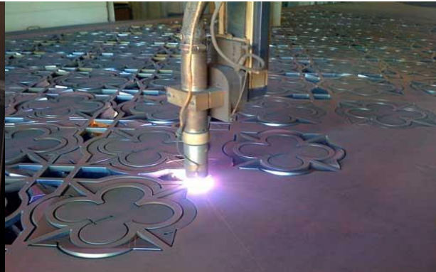
Figure 5 Cutting using a mechanical device
