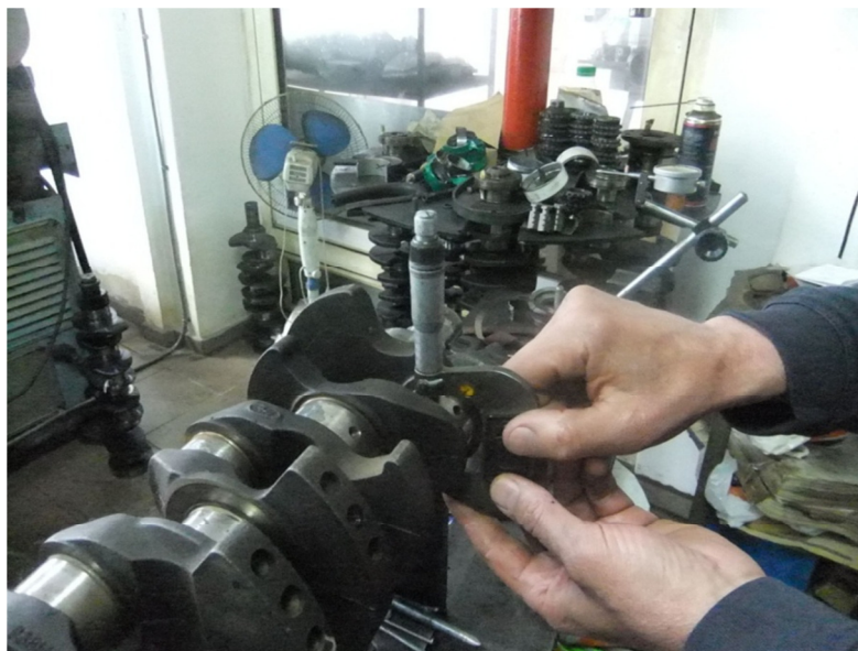
Figure 2 The measurement of oval-shaping in the journals of a main shaft in a Renault engine
