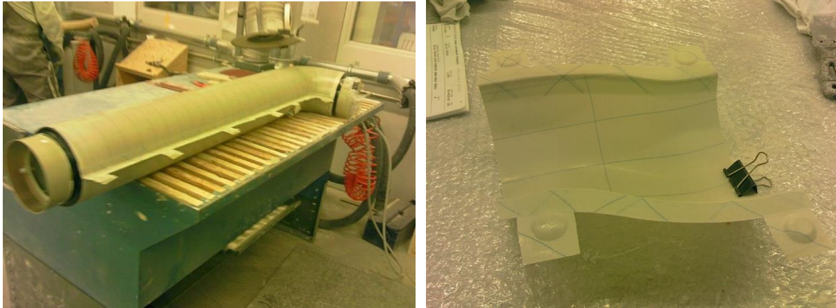
Figure 1. Air duct for an Airbus air conditioning system.
