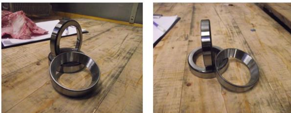
Figure 5 Superfinished rings (left) and after stamping with ID characters (right)
