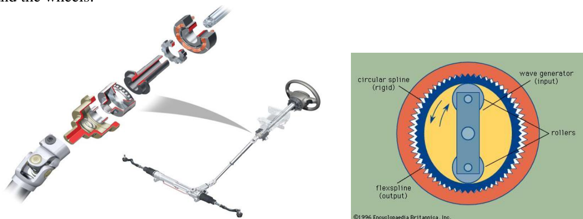
Figure 2 AUDI steering unit with harmonic drive [1]
