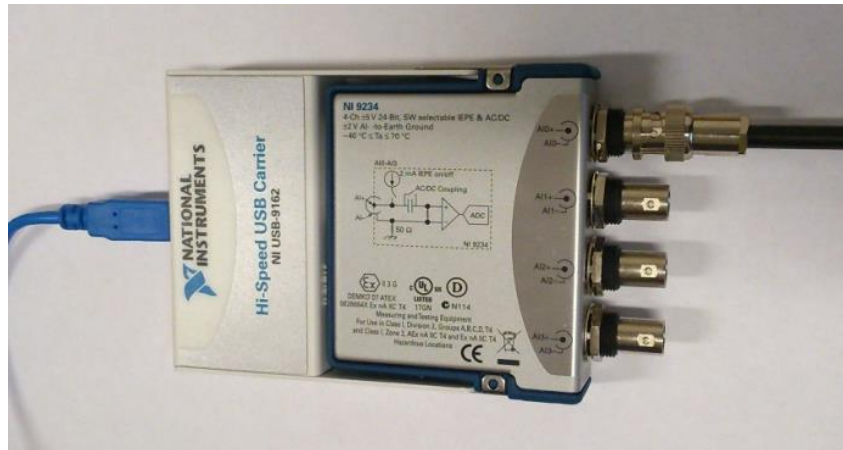
Figure 4 NI USB-9234 data acquisition (DAQ) module
