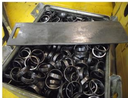
Figure 15 Storing box covered with rubber layer
