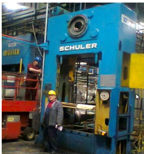
Figure 2 Press frame closed undergoing modernization; Analog electric panel.
