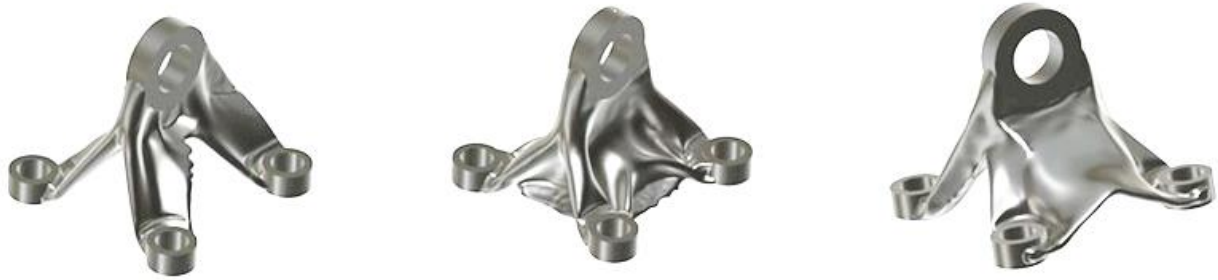
Figure 2 Results of the generative design process.
