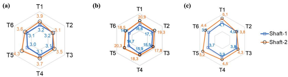
Figure 3 Comparison of the roughness amplitude parameters hinted at better manufacturing precision of Shaft-1; Polar plot of (a) average, (b) maximum, and (c) root-mean-square roughnesses of Shaft-1 and Shaft-2
