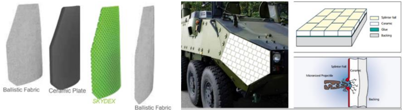
Figure 3 High-resilient technical ceramics (left: SKYDEX; right: composite armour system) [4]
