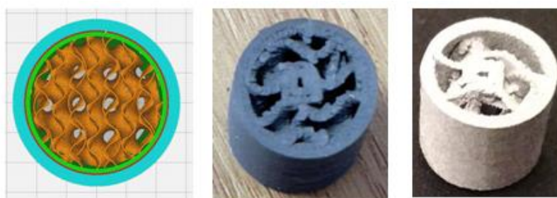
Figure 2 Additive fabrication steps a. -3D image; b.-printed part and c.- sintered part
