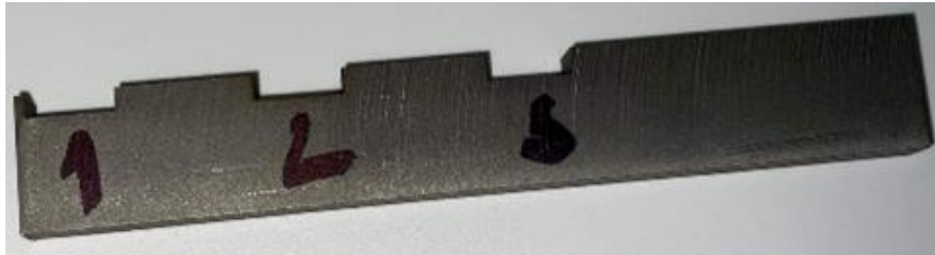
Figure 1 Carbide specimen machined through progressive electrical discharge machining technology
