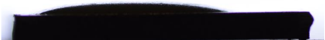
Figure 2 Good wetting behaviour of potting on aluminium sheet
