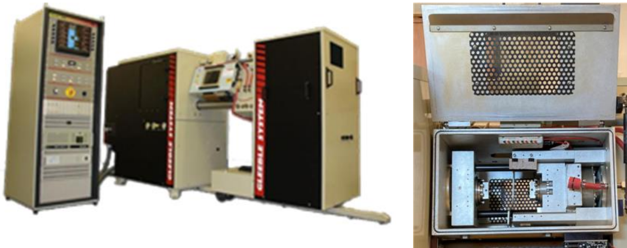
Figure 1 GLEEBLE 3500 thermo-mechanical simulator and the testing space
